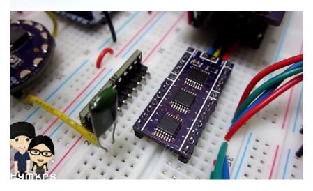
Assembled PCB on Breadboard gating 8 555-based signals!
